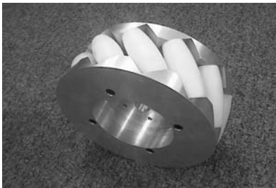
Figure 8.1: Mecanum wheel designs with rollers at 45^\circ
