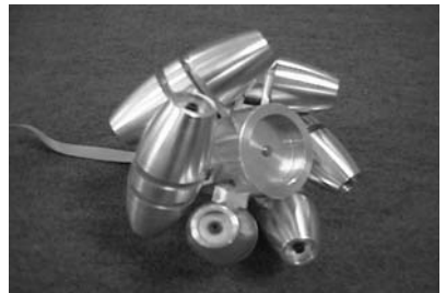
Figure 8.1: Mecanum wheel designs with rollers at 45^\circ
